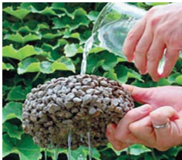
Figure 9.3 Water passing through pervious concrete (NRMCA 2009)
