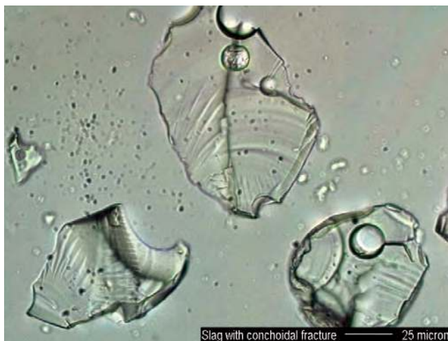
Figure 4.5 Petrographic optical micrograph of slag cement particles (image courtesy of CTLGroup)
