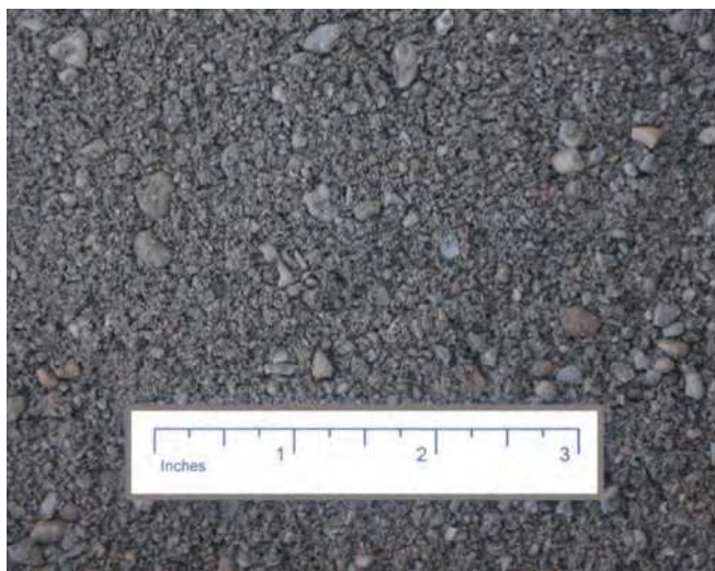
Figure 4.8 Light-weight fine aggregate (image courtesy of Buildex)
