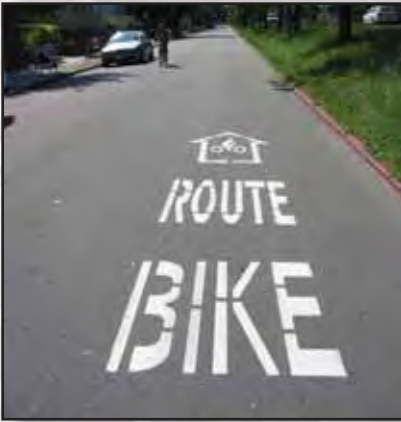
Separate facilities for bicyclists may be unnecessary on low-speed, low-volume urban streets.
