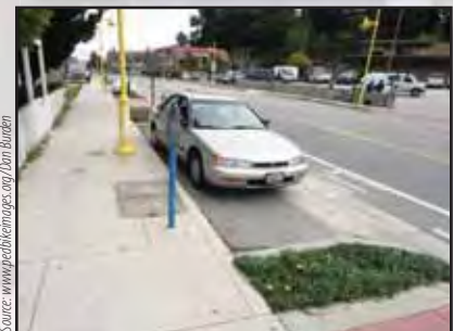
On-street parking located in 'pockets,' where the gutter pan is located to the left of the driver's side door.
