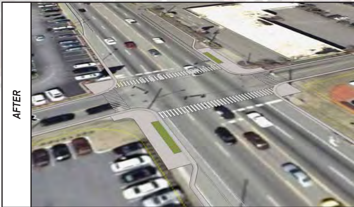
Curb extensions are a good strategy for making intersections more walkable.
