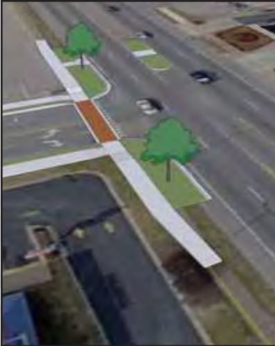
Aligning curb extensions with raised median islands is an effective, low-cost strategy for creating safe crossing opportunities.
