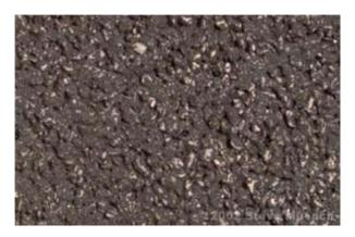
The development of open graded hot mixes was a possible solution to the problems associated with chip seal construction. These pavements have been shown to reduce hydroplaning and poor visibility from splash and spray.
