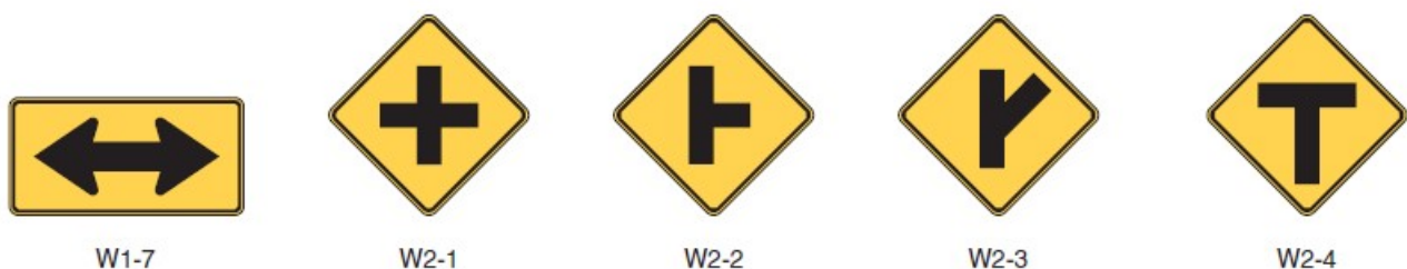
Figure 2C-9. Intersection Warning Signs and Plaques
