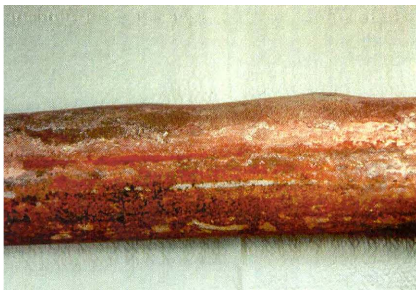
Figure 3-7. Metal Fatigue on Boiler Tube
