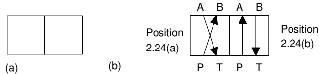
Figure 2.25 (a) The basic symbol for a two position valve, (b) the 4/2 valve
