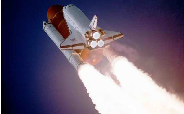
Each Space Shuttle is loaded with approximately 55 tons of propellant. AP makes up 70% of the fuel.
