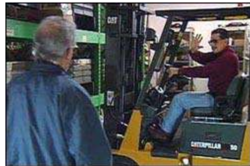
Figure 7. Operator signaling to coworker to stand back.
