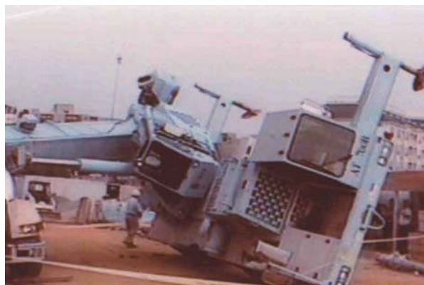
Figure 4. Crane tip-over at construction site. Note that the right outriggers were set, but not extended. (Photo courtesy of OSHA)
