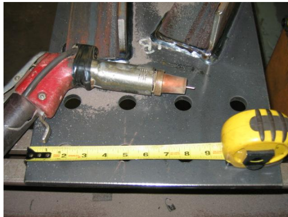
Figure 5 Photo of Submerged Arc Welding (SAW) equipment
