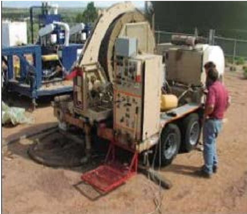
Figure 4-6: Coil tubing rig capable of 1500 foot hole developed by LANL.
