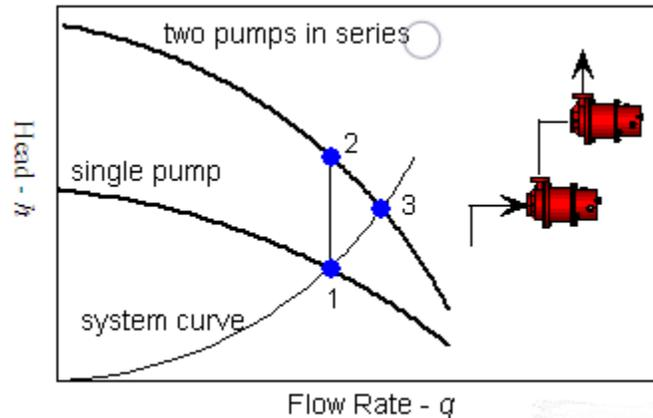
Fig. 1. Head for Two Pumps in Series.
