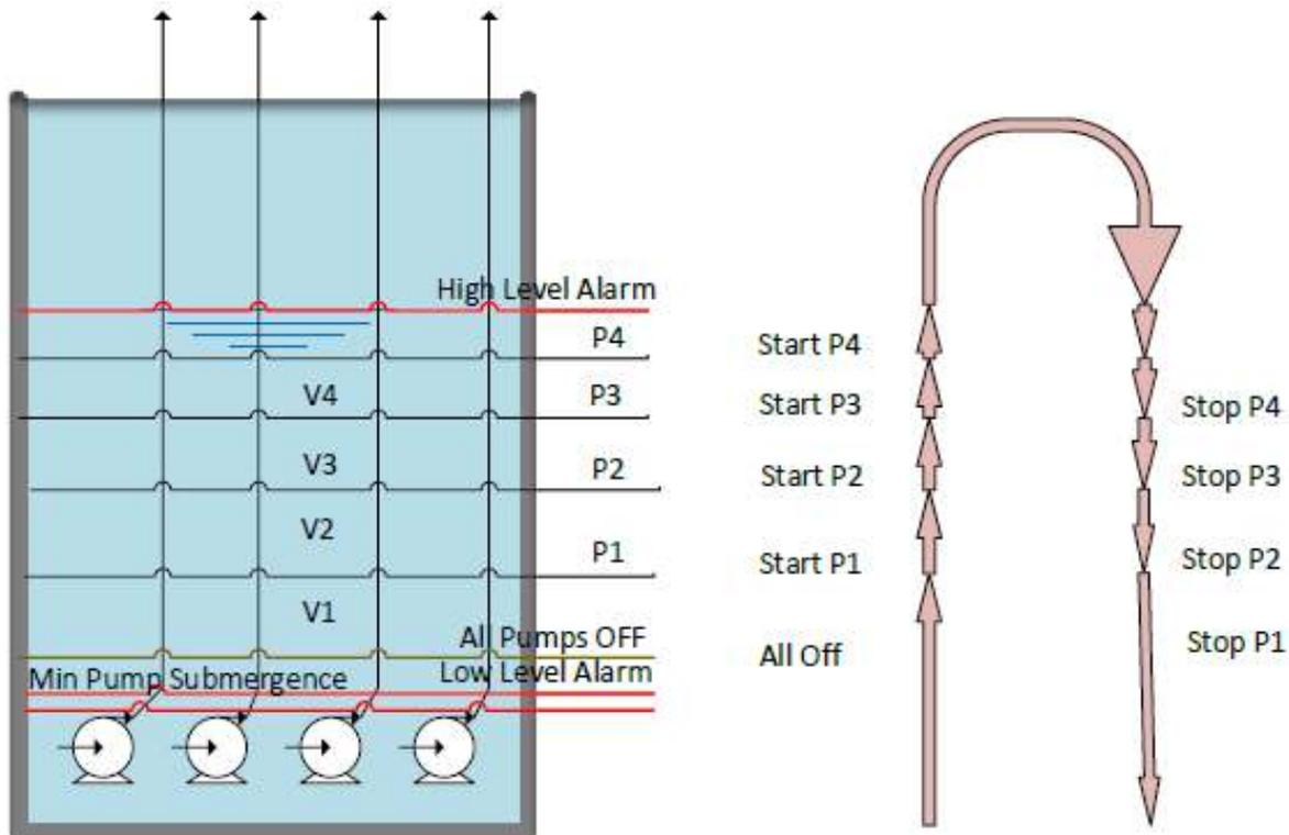
Fig. 9. Lift station with a 4-pump sequence.
