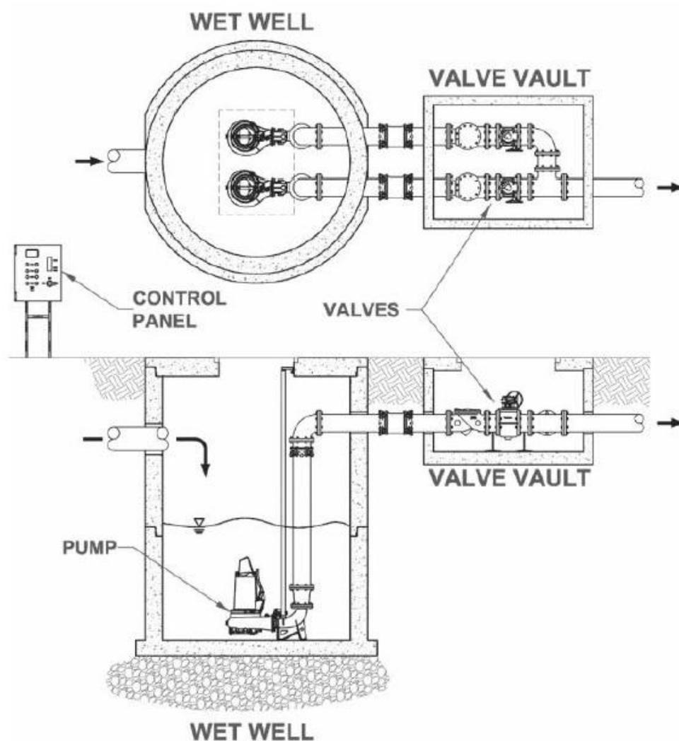
Fig. 4. Typical Duplex Submersible LS with Parallel Pumps.
