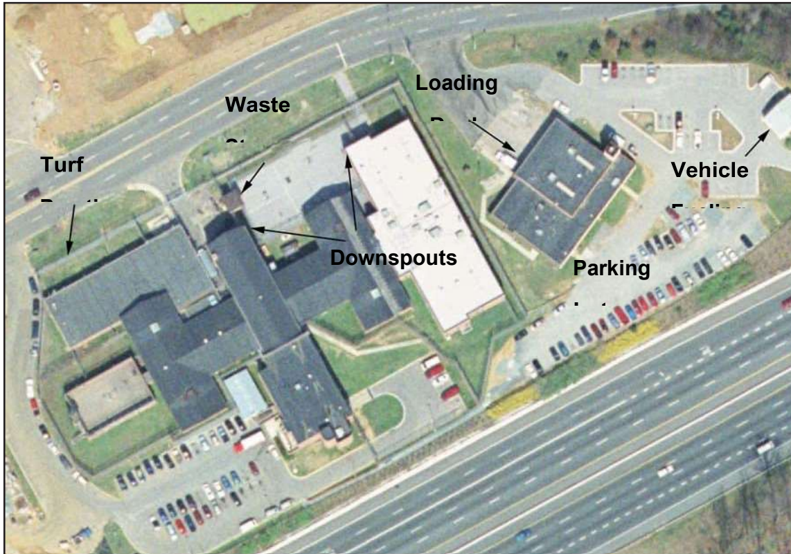
Figure 24: Investigating Potential Storm Water Hotspots
