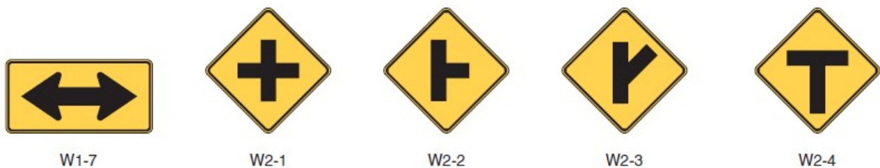
Figure 2C-9. Intersection Warning Signs and Plaques
