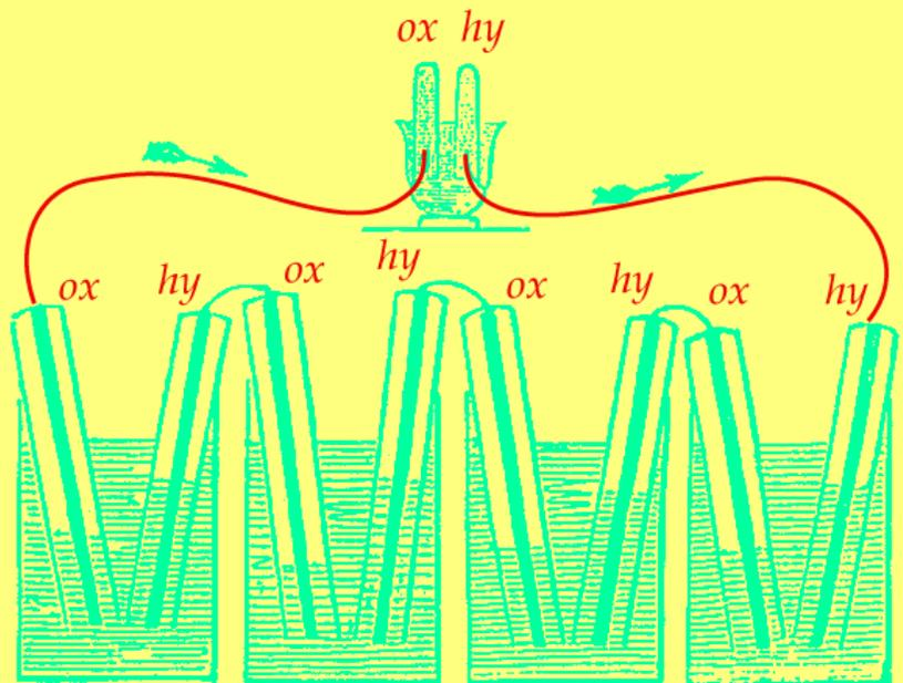
*In 1839, William Grove, a British jurist and amateur physicist, first discovered the principle of the fuel cell. Grove utilized four large cells, each containing hydrogen and oxygen, to produce electric power which was then used to split the water in the smaller upper cell into hydrogen and oxygen.*
