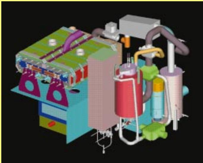
Computer model of 50kW fuel cell stack with reformer.
