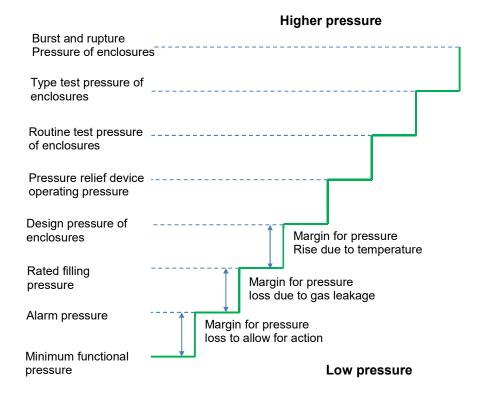
Figure 1. Pressure coordination of enclosures and pressure-relief elements
