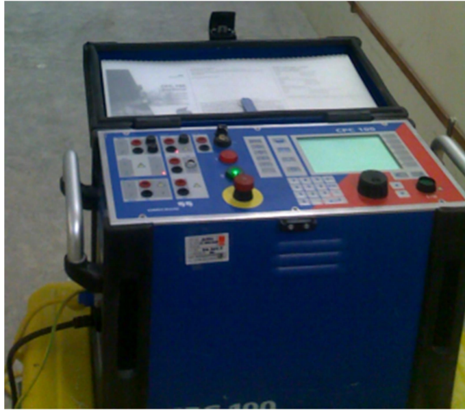
Figure 20. Modern PC-based secondary injection test equipment
