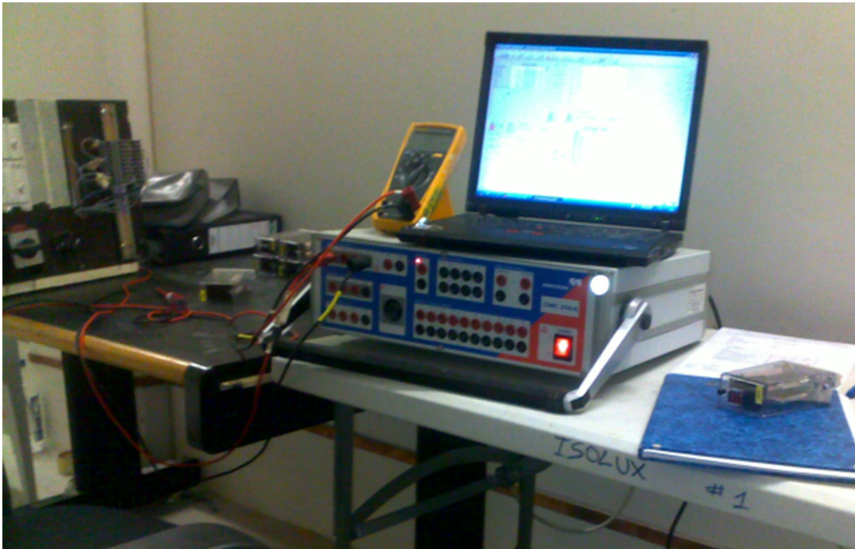
Figure 14. Modern computer-controlled test bench
