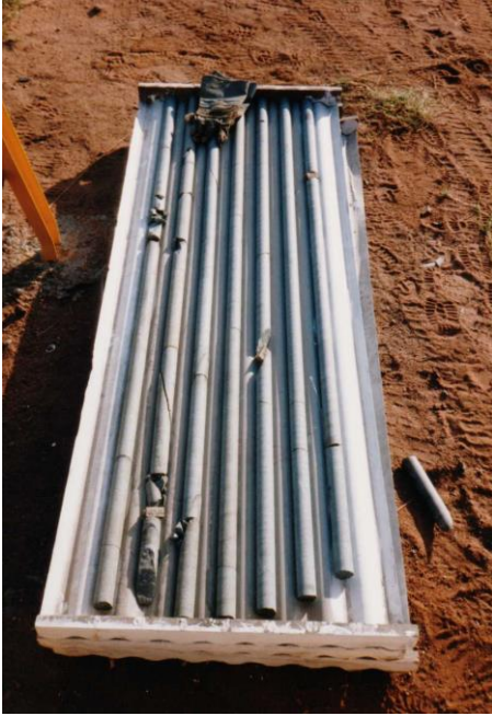
Figure 21: Excellent quality core with very few discontinuities from the massive gneiss of the Rio Grande project in Argentina.
