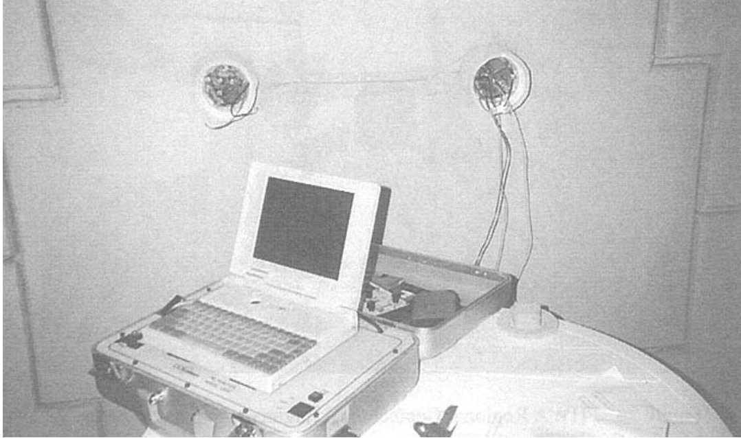
Figure 3-5. PR Monitor evaluation of a test location. Note horizontal adjacent access holes for cross testing.
