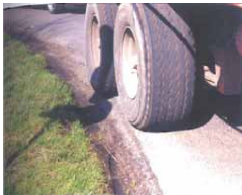
Figure 115: Edge loading conditions.
