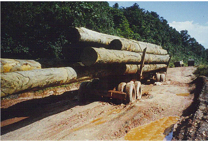
Figure 15: Timber truck completely stuck on an earth road due to too high contact pressures and a too low shear resistance of the pavement material.
