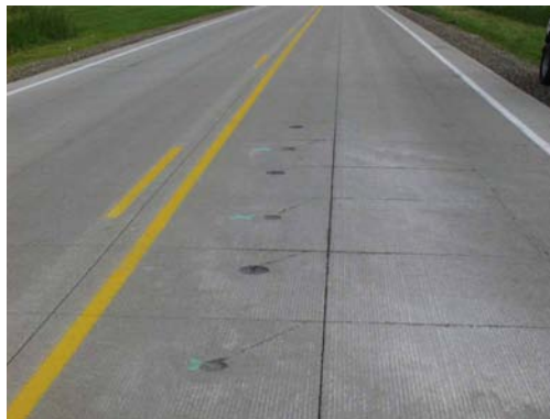
Figure 10. Temperature and strain gages along Iowa highway 13
