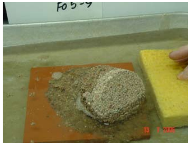
Figure 45B-4 Vaughan and Soares test on sample with good self-healing characteristics. As sample is submersed, capillary stresses are reduced and sample collapses quickly.
