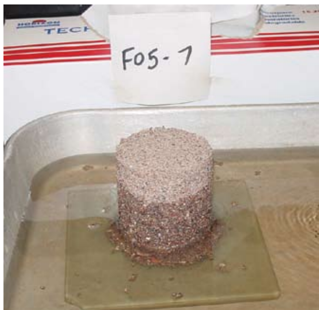
Figure 45B-3 Vaughan and Soares test on sample with poor self-healing characteristics. As sample is submersed, capillary stresses are reduced and sample should collapse. This sample does not collapse on wetting, demonstrating poor self-healing characteristics.
