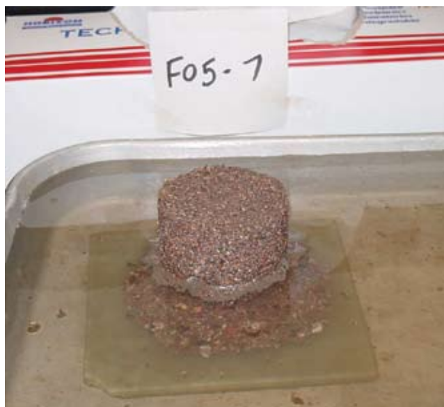
Figure 45B-3 Vaughan and Soares test on sample with poor self-healing characteristics. As sample is submersed, capillary stresses are reduced and sample should collapse. This sample does not collapse on wetting, demonstrating poor self-healing characteristics.
