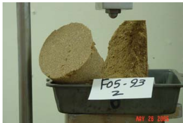
Figure 45B-5 Compressive strength specimen
