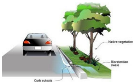
Fig. 18: Curb cut schematic
